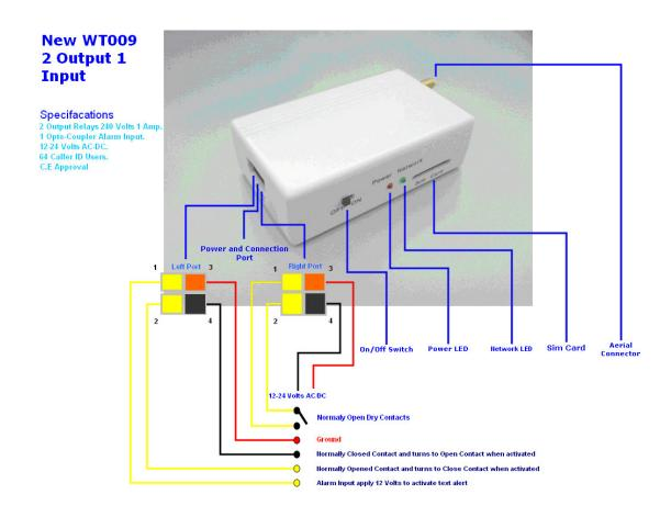
**EST-64 GSM Remote Control Device Diagram**
