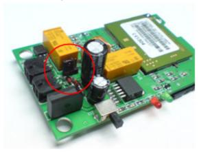
**Note:** Relay 2 will supply DC voltage only according to the output DC voltage of adapter used. When 24VAC adapter is used, the voltage supplied would be 33VDC.
